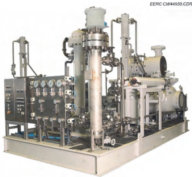
Figure 48. CryoStar turboexpander and demethanizer.
